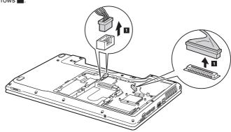
When installing: Make sure that the connectors are attached firmly.
